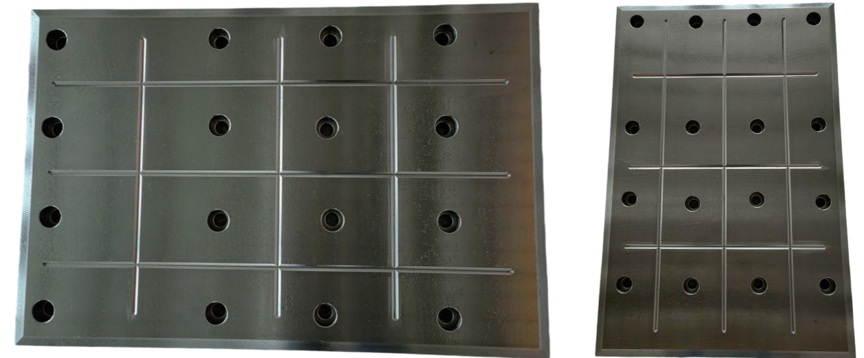
Finished product image of laser fusion bonding of the slide plate of the finishing mill
